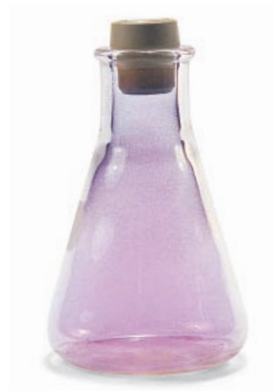
FIGURE 17-8 Clear hydrogen iodide gas, HI, decomposes into clear hydrogen gas and violet iodine gas.
