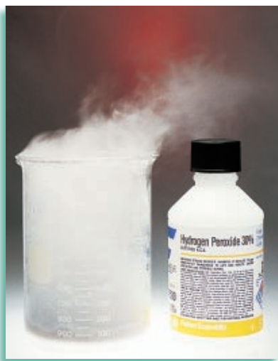
FIGURE 17-14 The reaction rate of the decomposition of hydrogen peroxide, \text{H}_2\text{O}_2 , can be increased by using a catalyst. The catalyst used here is manganese dioxide, \text{MnO}_2 , a black solid. A 30% \text{H}_2\text{O}_2 solution is added dropwise onto the \text{MnO}_2 in the beaker and rapidly decomposes to \text{O}_2 and \text{H}_2\text{O} . Both the oxygen and water appear as gases because the high heat of reaction causes the water to vaporize.
