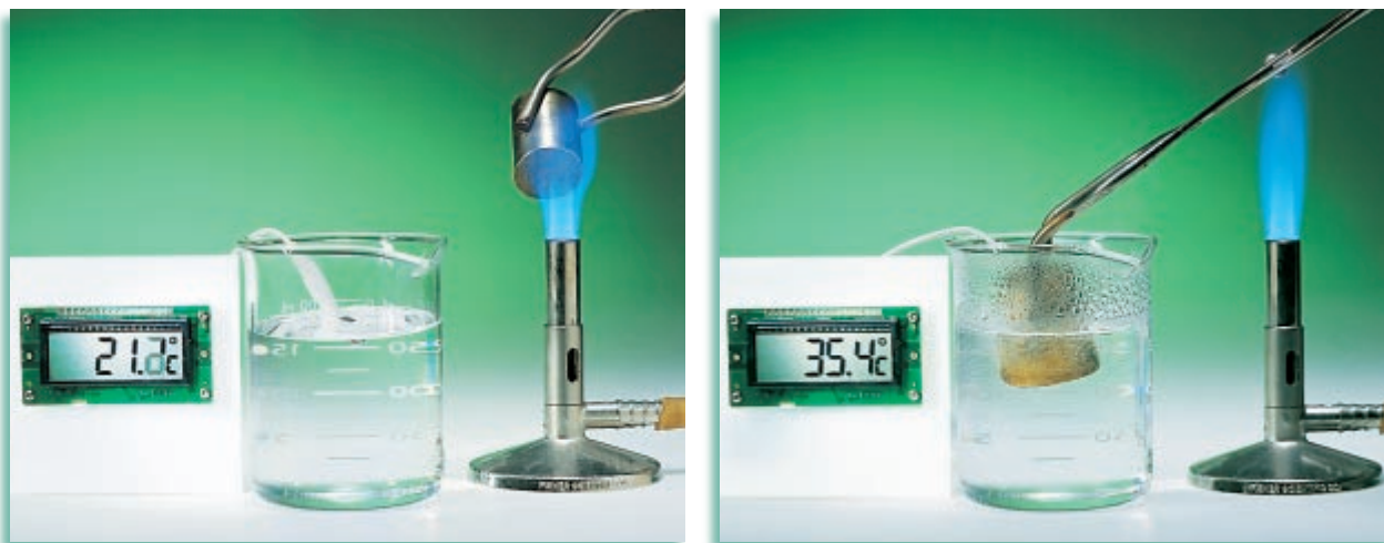
FIGURE 17-1 The direction of energy transfer is determined by the temperature differences between the objects within a system. The energy is transferred as heat from the hotter brass bar to the cooler water. This energy transfer will continue until the bar and the water reach the same temperature.
