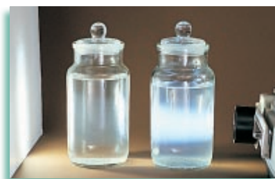
FIGURE 13-4 A beam of light distinguishes a colloid from a solution. The particles in a colloid will scatter light, making the beam visible. The mixture of gelatin and water in the jar on the right is a colloid. The mixture of water and sodium chloride in the jar on the left is a true solution.
