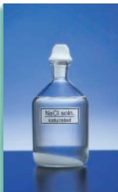
FIGURE 13-7 A saturated solution in a closed system is at equilibrium. The solute is recrystallizing at the same rate that it is dissolving, even though it appears that there is no activity in the system.
