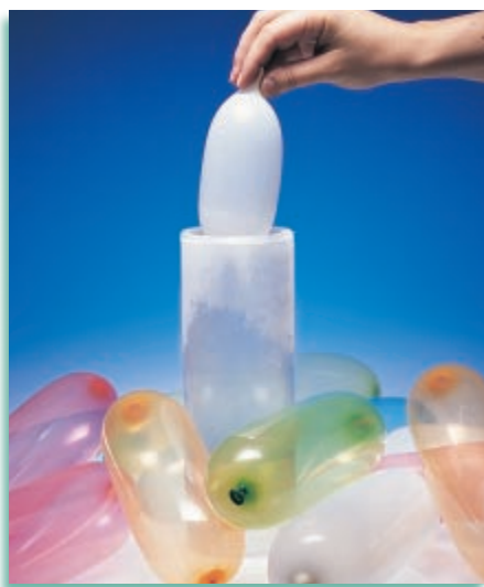
FIGURE 10-11 As air-filled balloons are exposed to liquid nitrogen, they shrink greatly in volume. When they are removed from the liquid nitrogen and the air inside them is warmed to room temperature, the balloons expand to their original volume.
